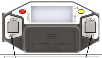
Press and hold both to remove from hold and return to measuring mode
