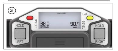
32. Holding the CJ4000 in position, press the HOLD LEFT or HOLD RIGHT button. Pressing the HOLD RIGHT button will show a display similar this.
