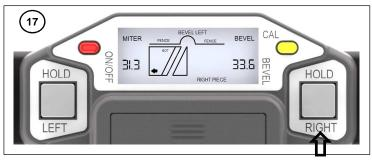
Note: you can press either of these buttons as many times as you want to switch the graphic from the left piece to the right piece. You can move the protractor arms to any position without losing the values. These values are held until you return to the measuring mode.
