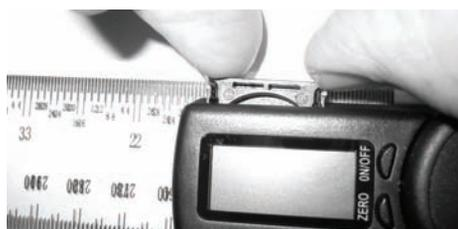
Pull the holder completely out of the protractor
